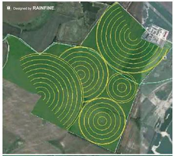
For maximum covering the land by center pivot, the circles can be designed in any angles to avoid the obstacles.
