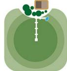
When the obstacle is inside the circle, the corner system can avoid the obstacle and maximize the field coverage.
