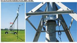
End gun and corner angle switch on/off.
