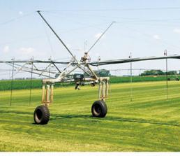
The steerable corner system is used to irrigate the four corners of the square and maximum the irrigation area. The last span can be extended to the maximum length in the corner and folded in the retracted position. The corner pivot consists a 6-5/8" diameter by 61.3m or 54.5m long span with an 26.8m overhang. When the corner span is fully extended, it will add 85m or 78m to the overall length of the main system. This system has a high cost.
